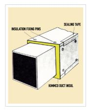
Carefully position insulation over the pins, pressing firmly so that pins penetrate through the insulation. Fit spring clip or lock washer over pins pushing them down until tight against insulation. Snip off any excess shank from pin. Seal all joints and openings with self adhesive tape.
